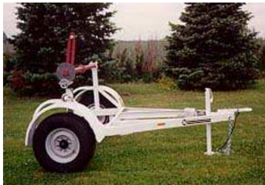
Trailer shown with optional over spin brake
